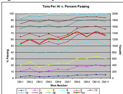
This chart shows the change in tons per hour to the crusher as well as the changes in the overall fragmentation from blast to blast.
