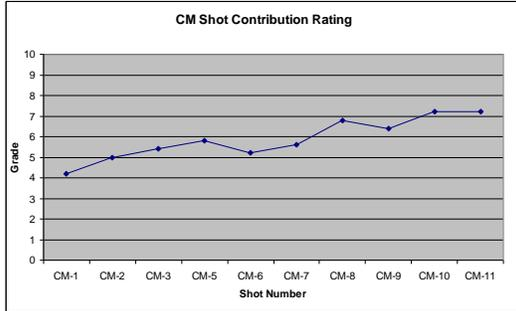
Based upon the contribution rating of a particular blast adjustments to the contributing factors for the next blast may be made in order to get the desired result. If for instance greater production rates are required, a blast design that will yield the desired fragmentation can be chosen.
